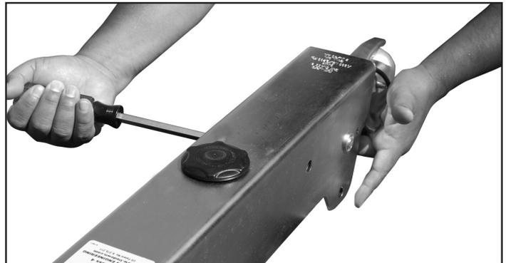
**While pressing the E-stop release, pump the master cylinder with your right hand 4 to 5 times.**
